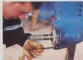
Replace the prop shaft and bearing. Fit a new anode and refill with oil.
