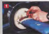
Having cut the locking wire, you can start undoing the studs. Note their positions.
