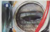
8 The rear of the gearbox and the gearbox plinth waiting for the leg and new seal.
