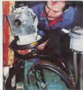
Engine has been eased forward (above) leaving a gap between the bell housing and the gearbox, disengaging the drive shaft, allowing removal of the leg and gearbox (right).
