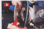
Separating the clamp plate and seal from the gearbox. Note the old 'O' ring on the clamp plate.
